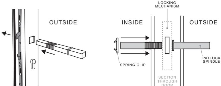
Hold the PATLOCK spindle firmly from the outside and push the spring clip onto the PATLOCK spindle from the inside of the door ensuring that the clip engages with the grooved section to secure in position.
